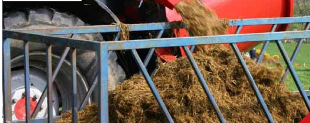
Independently hydraulic driven drum gives you better control over the feed rate of the bale, as you have more control over the hydraulics of the tractor than the PTO shaft.
