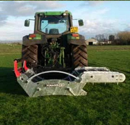
The Forager X10W is designed to unroll a bale into a trough or over a barrier or other obstacle. This model is based on the Forager X10, with the extension wing allowing silage, straw or hay to be dispensed further away.
