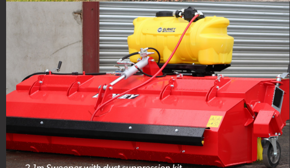
2.1m Sweeper with dust suppression kit
