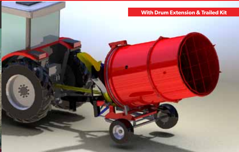
Rotor flow on straw provides a more even particle distribution over a greater distance
